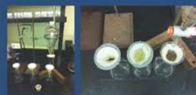
Fig. 4. Heavy mineral separation prior to color separation.
