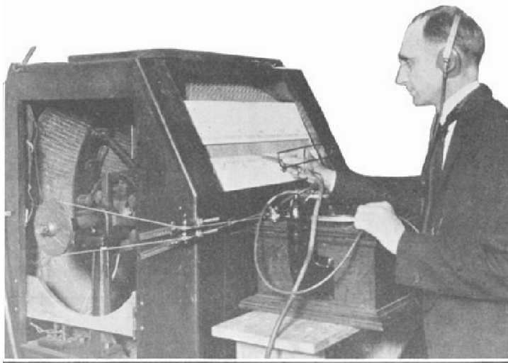
The tonoscope for analyzing the pitch of the tones on a disk phonograph record
