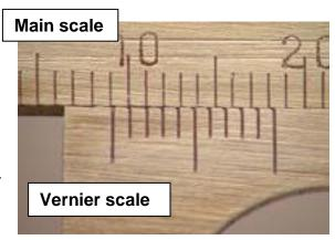
To use the Vernier scale, read the main scale to the last certain digit. The last certain digit on the main scale is the graduation just below the zero on the vernier scale. The mark on the vernier scale that directly lines up with a graduation mark on the main scale is the last digit in your reading.
